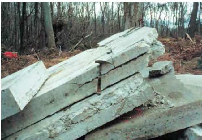
Figure 10. Horizontal cracking plane in CRCP.
